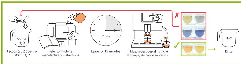
1. Add 1 scoop (25g) to 500mL of water and dissolve to form an orange solution. Pour into water tank (If machine has a water filter, remove this prior to turning machine on).
